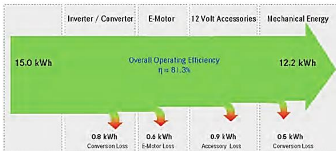
Figure 1 EV Operating Energy Flow and Efficiency Diagram (Source: Abdul-Hat et al. [59])
